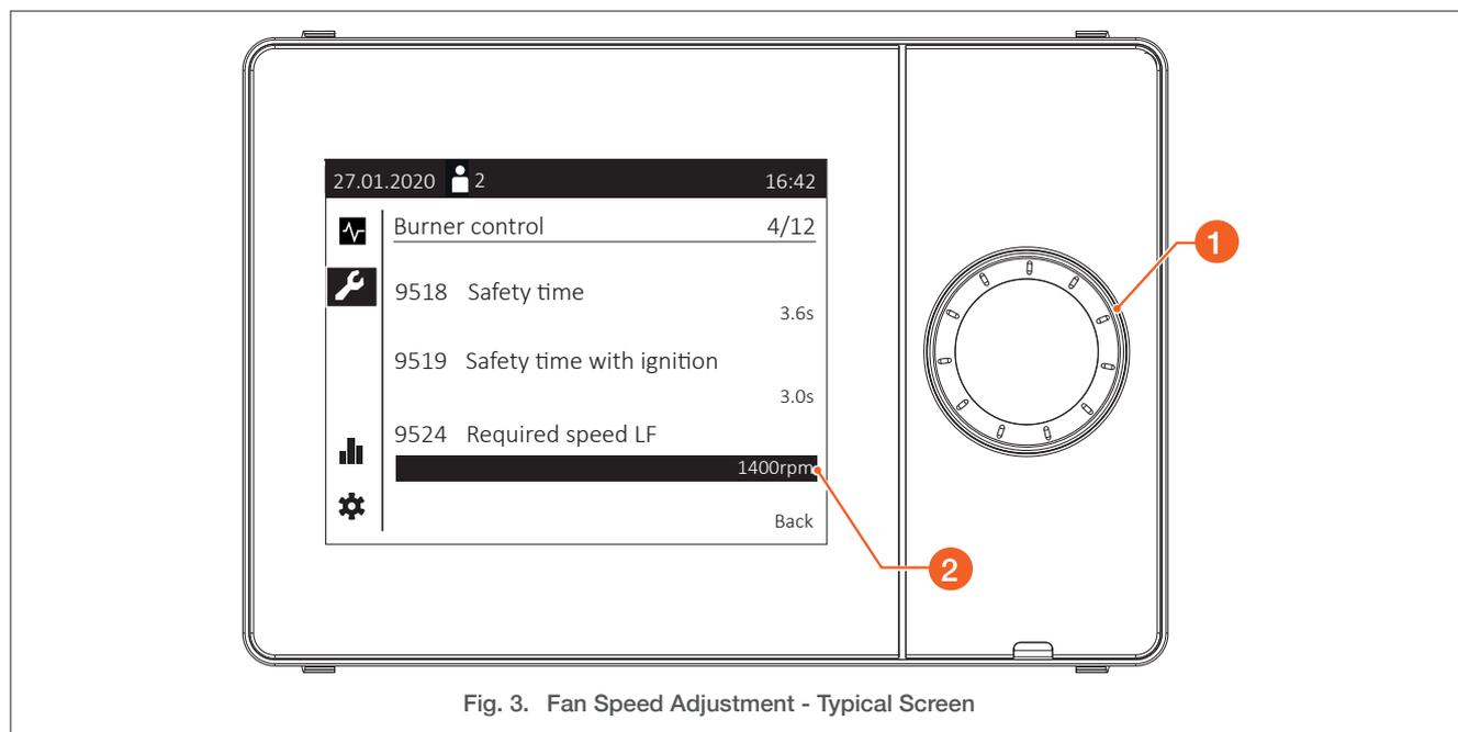
Fig. 3. Fan Speed Adjustment - Typical Screen
