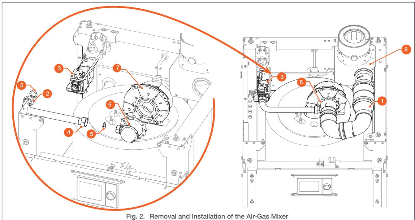
Fig. 2. Removal and Installation of the Air-Gas Mixer
